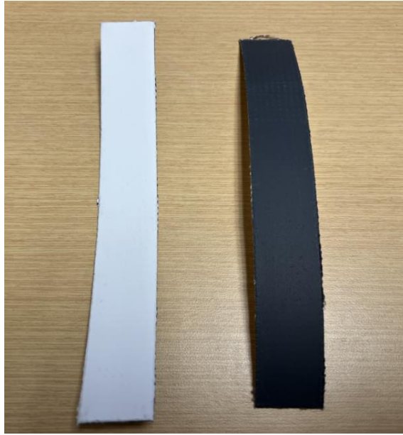
Figure 14 Samples of TPO membrane [32]
