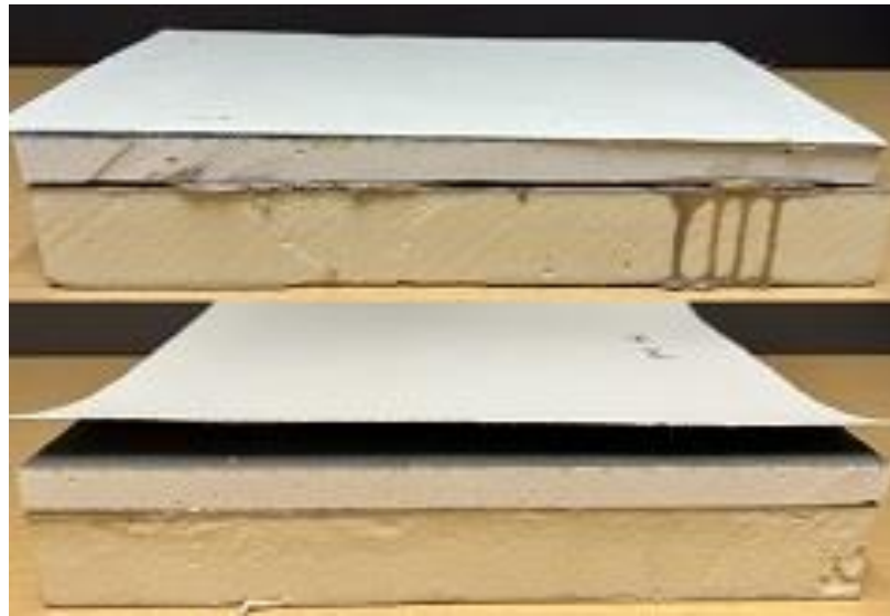
Figure 18 Fully-adhered (top) and non-adhered samples (bottom)
