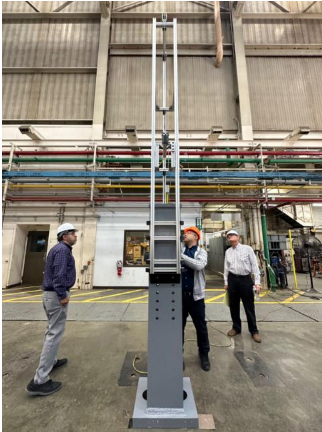
Figure 12 The drop tower ready for its first test
