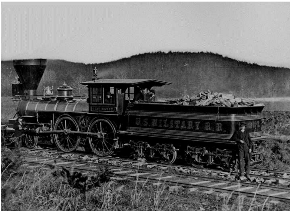
Fig. 17 - USMRC Crewman Posing Next to 4-4-0 "General Haupt," circa 1863, National Archives. A 4-4-0 Had Four Leading Wheels, Four Driving Wheels, and Zero Training Wheels. Nearly Every Railroad in North America Used Them in the 1860s.
