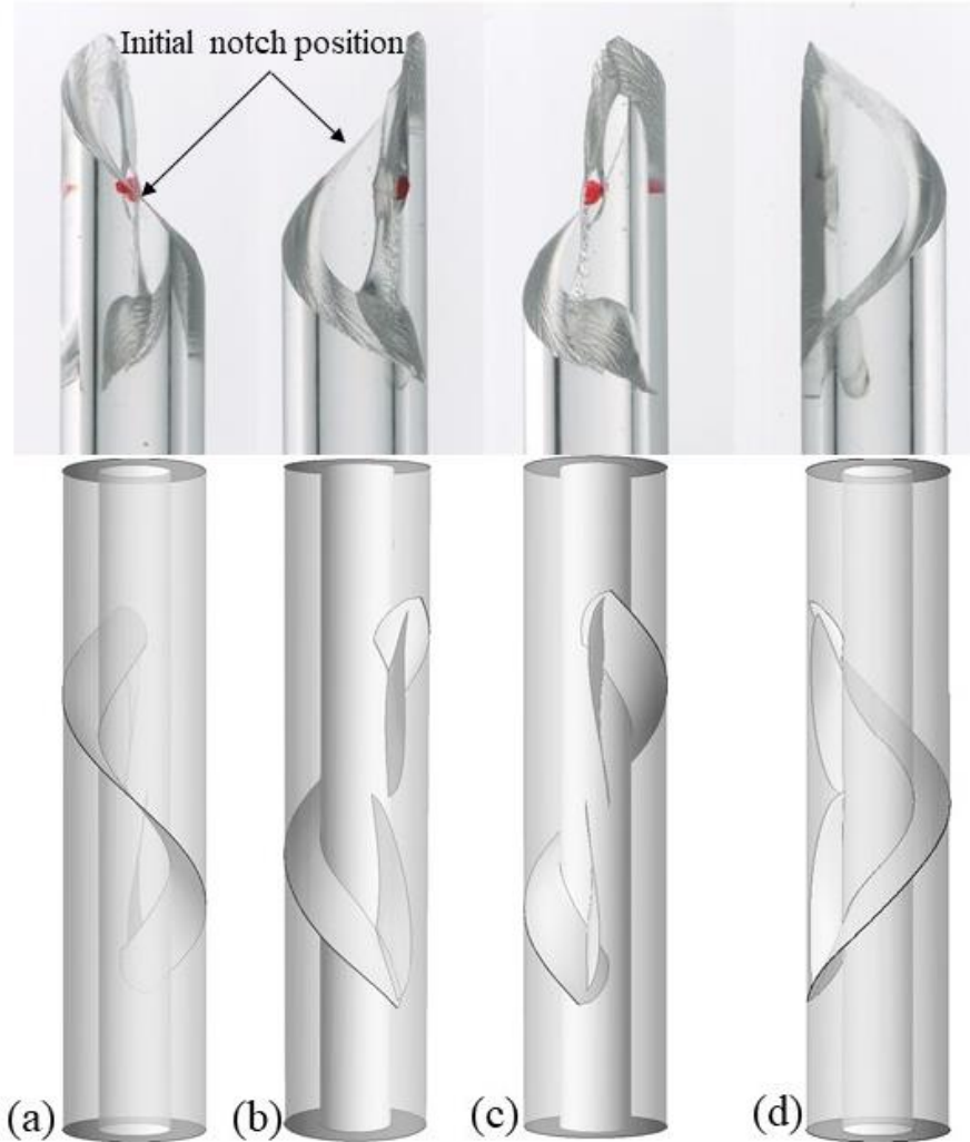
Figure 45. Comparison of experimental fracture surfaces for hollow cylinder ( r_1/r = 0.5 ) subjected to pure torsion with crack growth simulations.
