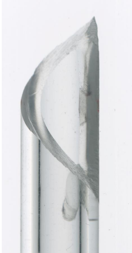
Figure 29. PMMA hollow cylinder fracture surface (pure torsion). r_1/r = 0.5
