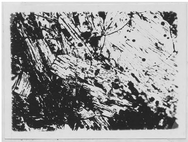
Fig. 30. Be-settled magnesium after immersion in 0.042 N HCl (1364 r.p.m. and 25°C) at an applied anodic current density of 0.07 amp./sq.cm. At this current density a dark precipitate is formed, and the attack on the surface becomes irregular. 375 X.
