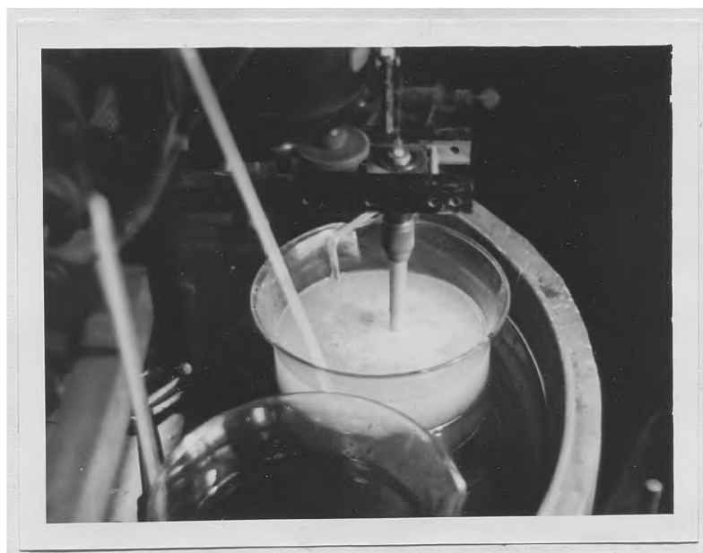
Fig. 20. Magnesium dissolving in 1.5 N HCl containing 0.5 mol/liter of \text{AlCl}_3 (1364 r.p.m. and 25^{\circ}\text{C} ). The hydrogen bubbles are small, giving diffuse reflection of light.
