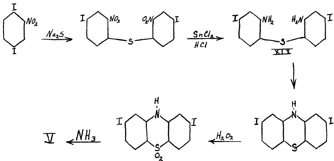
The reactions proceeded satisfactorily up to the ring closure of 2,2'-diamino-4,4'-diiododiphenyl sulfide (XIX). Ring closure of this compound by heating the monohydrochloride and by heating the tin complex (7, 22) both failed. These findings are in agreement with those of Matsumura (28) who found that 2,2',4,4'-tetraminodiphenyl ether could not be cyclized either by heating the hydrochloride alone or with zinc chloride.
