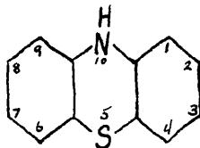
In direct electrophilic substitution reactions, directive influences of the ring nitrogen overshadow those of the sulfur, in most cases. Thus, the direct nitration of phenothiazine with nitric acid leads first to 3-nitrophenothiazine-5-oxide (9, 10, 24), with stronger acid to 3,7-dinitrophenothiazine-5-oxide (9, 10) and by heating with strong acid to 1,3,7,9-tetranitrophenothiazine-5-oxide (5).
