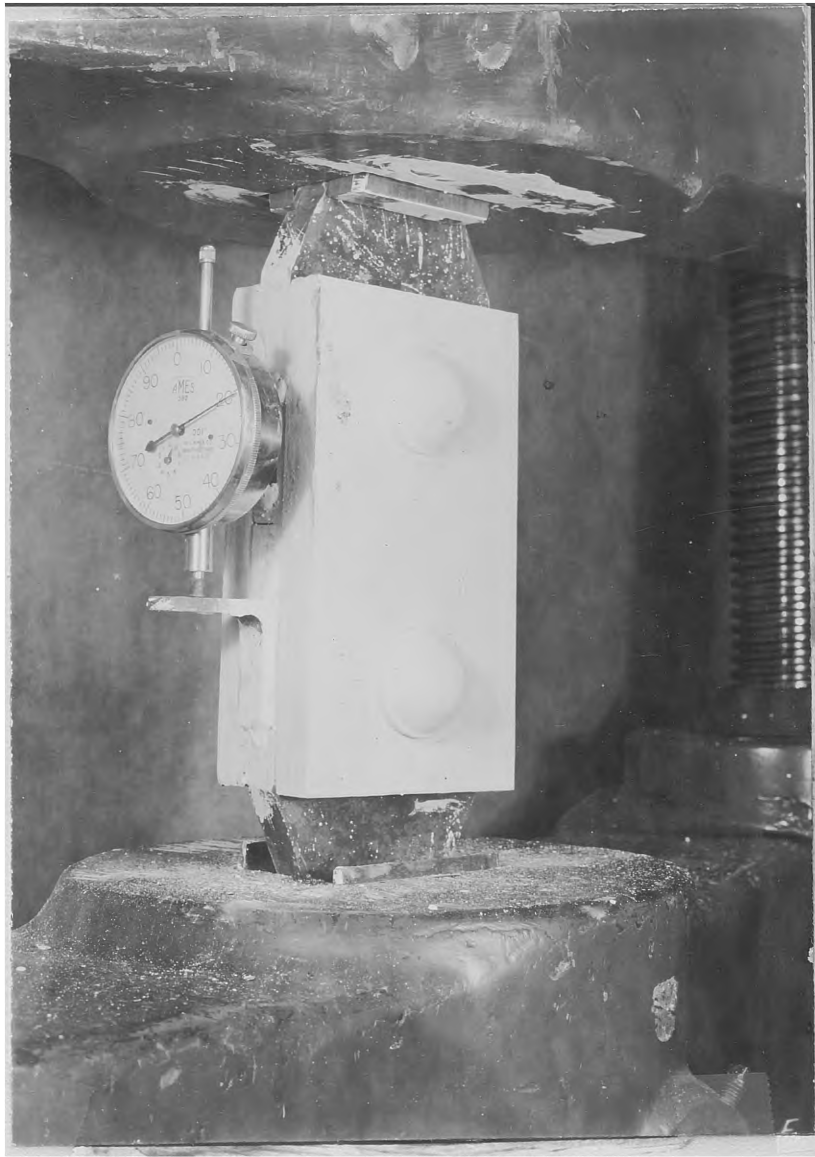
Fig. 18 Test of Riveted Joint
