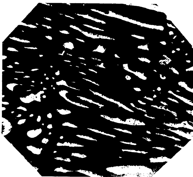
Plate 2. Eutectic-like intergrowth of pyrrhotite (gray) and silver (white) resulting from crystallization of a pyrrhotite-rich liquid. The charge ( 50\text{Ag} + 50\text{FeS} ) was annealed at 1010 \pm 5^\circ\text{C} for 20 minutes prior to quenching. (x 510 oil)
