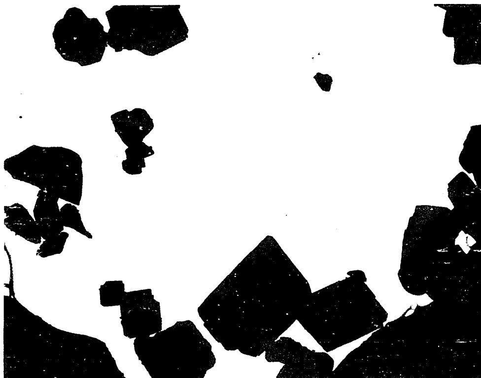
D. STARTING ALLOY POWDER. 8.23 ATOMIC PERCENT LITHIUM ALLOY. 2357X. ONE INCH EQUALS 10 \mu .
