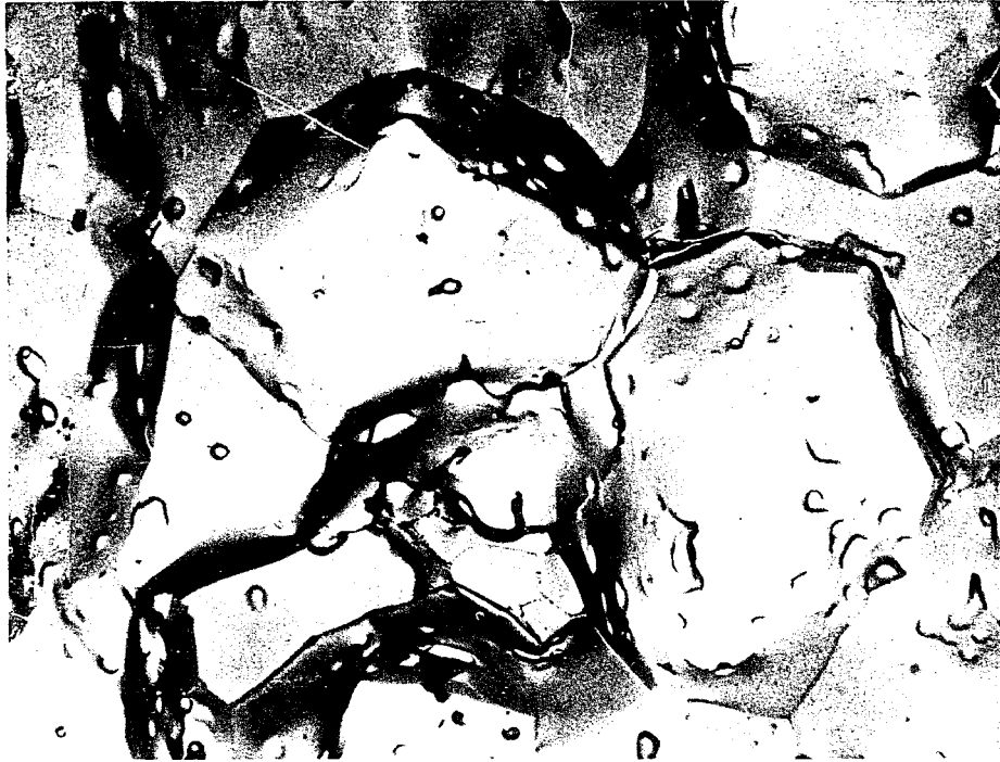
C. CARBON-CHROME REPLICA OF 1.96 ATOMIC PERCENT LITHIUM ALLOY. 2839 X. ONE INCH EQUALS 10 \mu .
