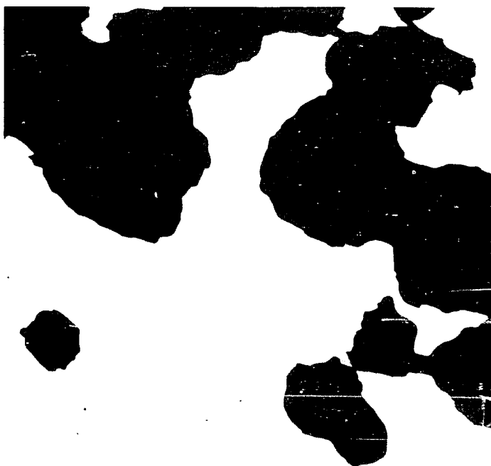
B. STARTING ALLOY POWDER. 0.12 ATOMIC PERCENT LITHIUM ALLOY. 2357X. ONE INCH EQUALS 10\mu .
