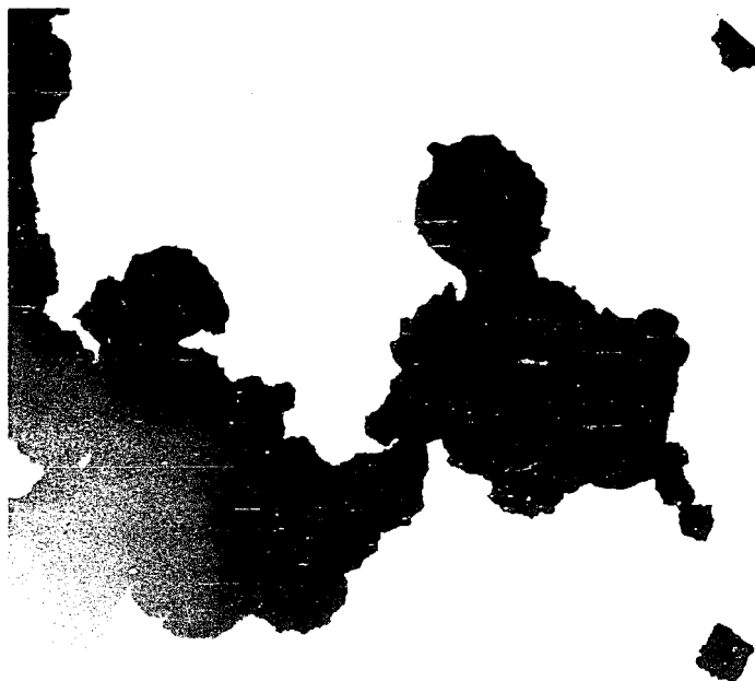
A. STARTING POWDER. PURE NICKEL OXIDE. 2300X. ONE INCH EQUALS 11\mu .
