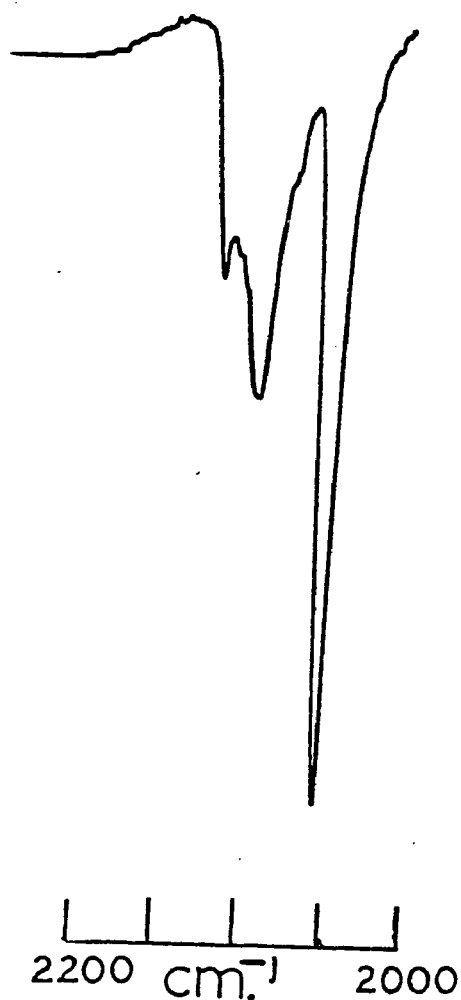
Figure 62. Infrared absorptions in the CN stretch region of [\text{Pd}(\text{dpp})(\text{NCS})_2] in Nujol.
