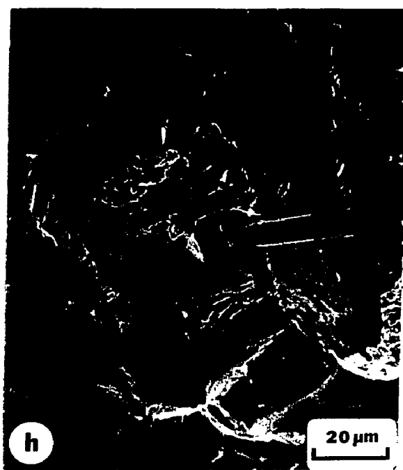
Low Stress. Near final failure
