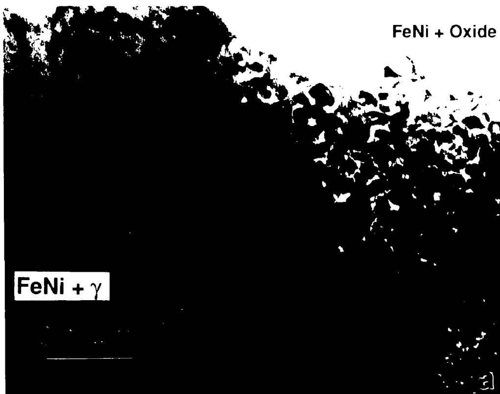
Fig. 4.33 a) TEM BF image of the USNM#3043 sample. A cloudy zone-like structure in the non-oxidized region labelled FeNi+ \gamma is observed. b) and c) \langle 110 \rangle_{\text{fcc}} zone axis electron diffraction patterns taken from non-oxidized (light regions in the BSE image) and oxidized (dark in the BSE image) regions showing the presence of ordered FeNi in both type of regions.
