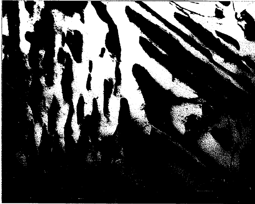
Figure 4.20 Pearlite in HAZ, showing lamellar microstructure and two pearlite colonies. Heat A, 5KJ/mm, PWHT 620°C/10hrs
