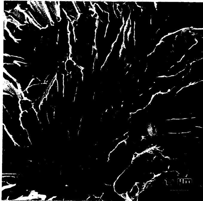
Figure 4.50 (a) Schematic fracture appearance of specimen A, showing crack initiation site and crack propagation direction (b) SEM fractograph of specimen A, tested at -49.9^{\circ}\text{C}
