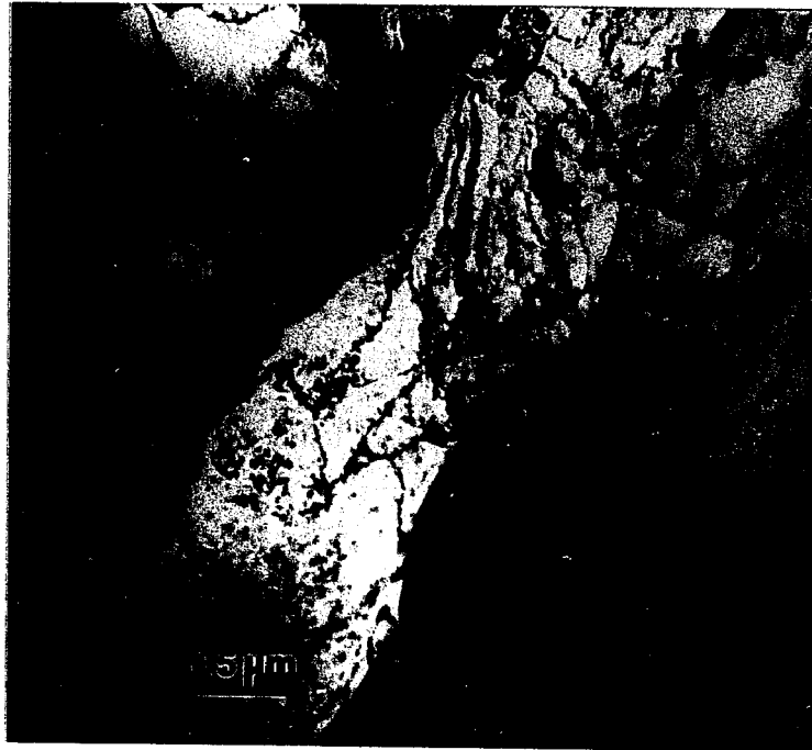
Figure 4.17 Intragranular Widmanstätten site ferrite, heat G, 3KJ/mm, PWHT at 620°C for 10hours
