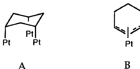
Figure 27. Possible Modes of Cyclohexane(A) and Cyclohexene(B) Adsorption on Pt(111) 99
