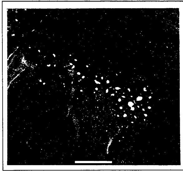
Figure 26. Lead segregation to eutectic nodule boundaries in Zn-5%Al-mischmetal alloy.
