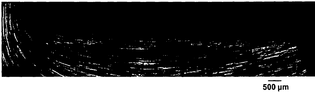
Figure 35: LOM collage from die face of low chromium sample 895 revealing dead metal zone and highly banded shear zone.
