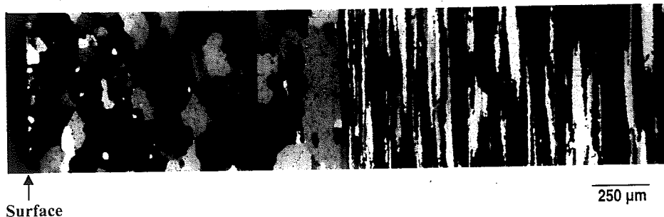
Figure 8: Aluminum 6063 alloy exhibiting common peripheral coarse grain layer at surface of extrudate.
