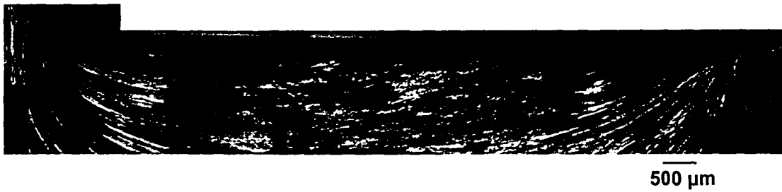
Figure 26: LOM collage from die face of sample 891 revealing dead metal zone and highly deformed grains within shear zone.
