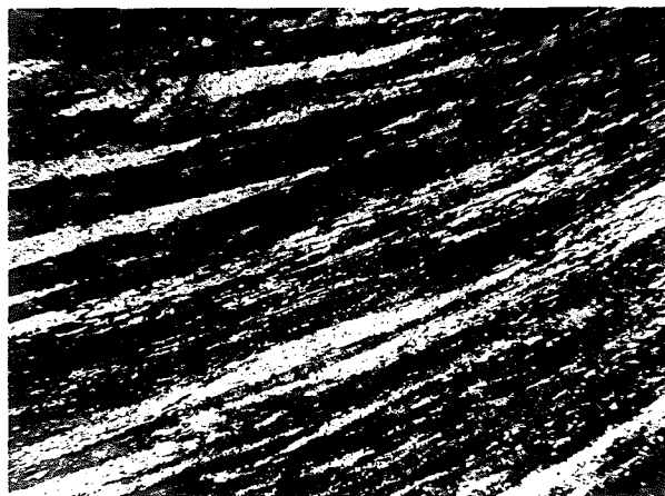
Figure 37: Image taken near die corner of extrusion discard for sample 883 revealing highly serrated and fragmented grains.
