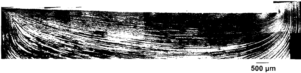
Figure 36: LOM collage from die face of low chromium sample 896 presenting dead metal zone and highly banded shear zone.
