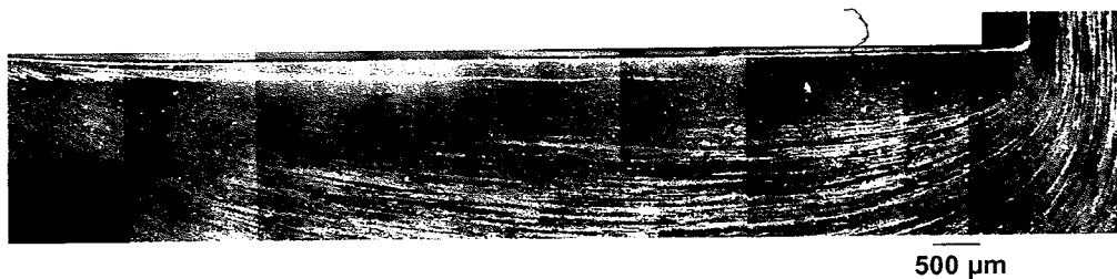
Figure 24: LOM collage from die face of sample 880 presenting dead metal zone and banded grains within shear zone.
