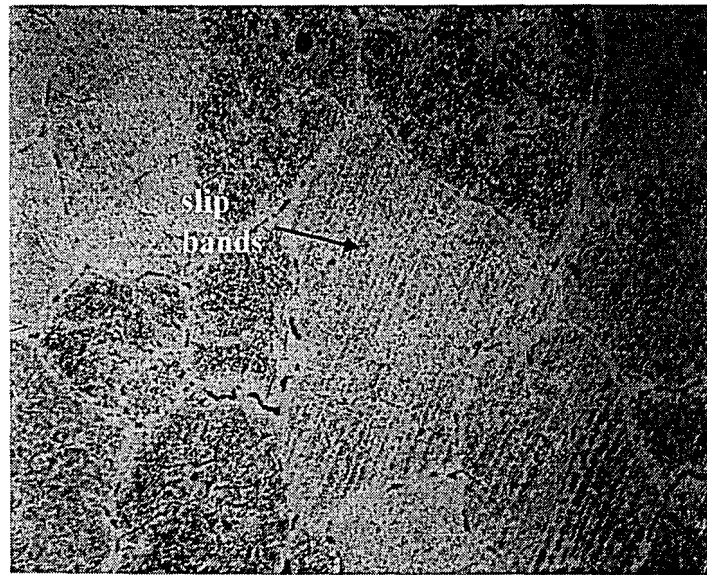
Figure 40: Magnified LOM image of slip bands in certain grains at the interface between Zone I and Zone II. (5% HF)
