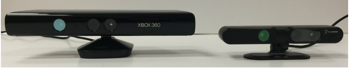
Figure 2.2: Examples of structured light based sensors. (Left) The Microsoft Kinect. (Right) The Primesense Carmine 1.09.
