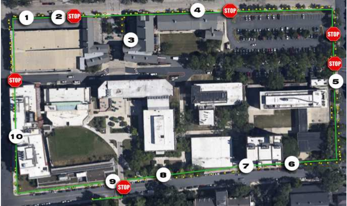
Figure 6.9: Satellite view of the block route network. The route is depicted as the green path. The yellow circles indicate the landmark features. The distance around the loop is approximately 944 meters. The six stop sign icons correspond to locations where the SWS automatically stops and waits for the operator to determine when it is safe to cross. The numbered locations correspond to labeled destinations for SWS navigation.
