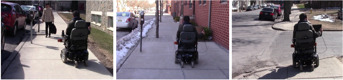
Figure 6.14: Photos of the SWS in operation, highlighting interactions with pedestrians (left), the narrowness and clutter of certain sidewalk areas (center), and automatically pausing at a crosswalk (right).
