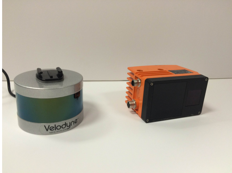
Figure 2.4: Examples of 3D LIDAR sensors. (Left) The Velodyne VLP-16 scanning LIDAR. (Right) The IFM O3D200 flash LIDAR.
