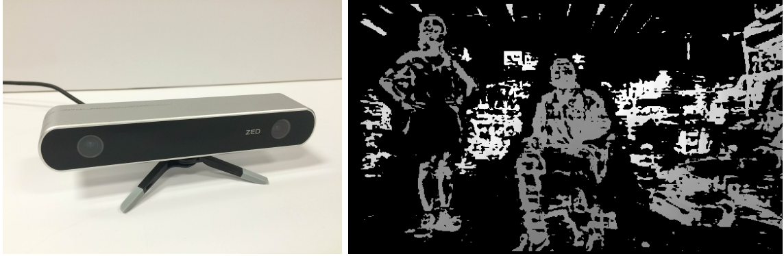
Figure 2.1: (Left) The Stereo Labs Zed stereo camera. (Right) A representative depth image captured by the Zed camera. Distance is colored on a grey to white scale where grey is nearer to the camera. Black pixels indicate that a point correspondence could not be found between the two camera images.
