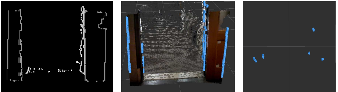
Figure 5.3: (Left) Edge image of doorway. (Center) Edge pixels identified in the scene. (Right) Top down view of door edge coordinates.
