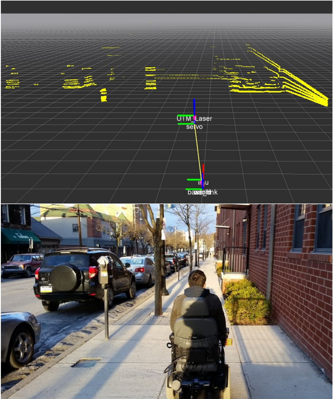
Figure 2.6: (Top) A scan from the 3D Hokuyo. (Bottom) A photo of the corresponding scene.
