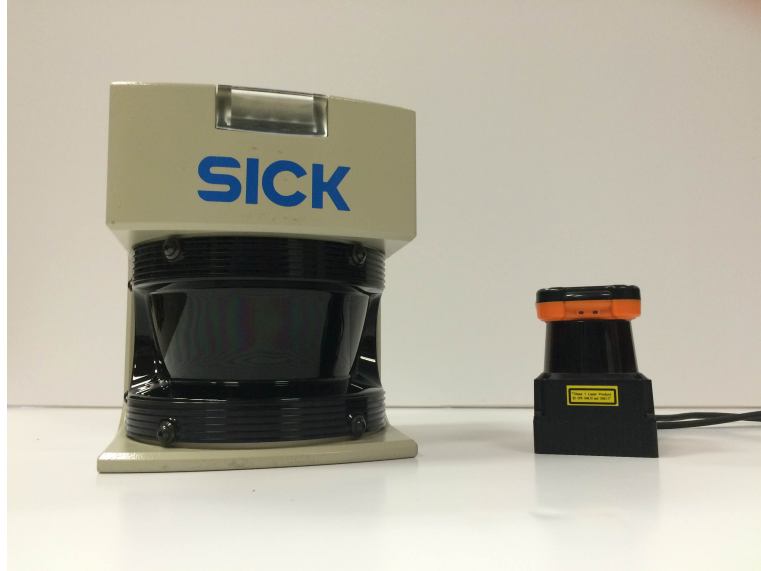
Figure 2.3: Examples of scanning LIDARs. (Left) The SICK LMS 291. (Right) The Hokuyo UTM-30LX.
