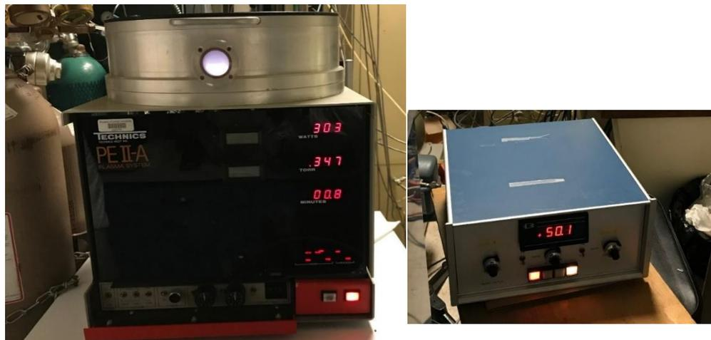
Figure 4-12: O<sub>2</sub> Plasma Ashing Machine.
