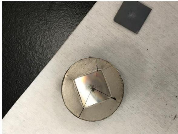
Figure 4-30: Zr-BMG TPF at 340C with 250 Kg.
