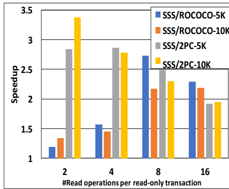
Figure 4.8: Speedup of SSS over ROCOCO and 2PC-baseline increasing the size of read-only transactions.
