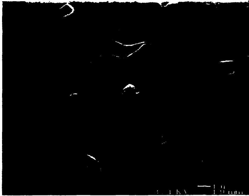
Figure 6. 17 Sub-surface region of AA5-5 at low indentation stress. No visible damage could be observed in the high shear region beneath the indenter.
