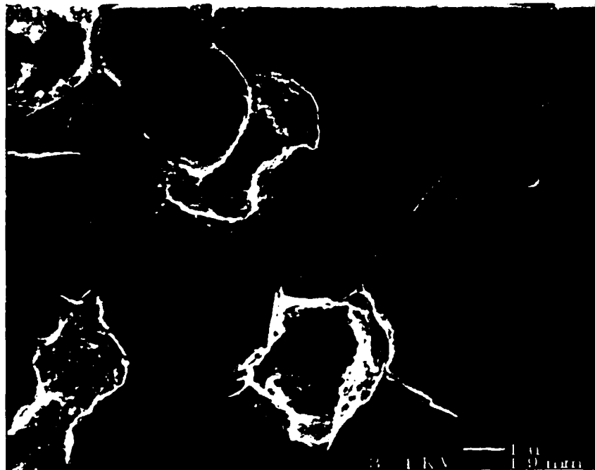
Figure 6. 18 Indentation of the AA5-5G sample at low indentation stress produced visible cracking within the microstructure in the high-shear region beneath the indenter.
