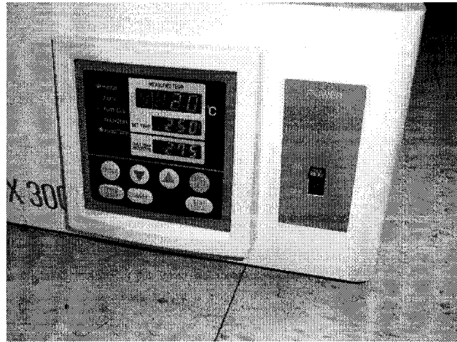
Figure 5.8: Front panel of the DX 300 oven where the temperature is set and monitored. Temperature is rigidly controlled and does not fluctuate when oven has reached set point. Over-temp control prevents overheating in case of microcontroller malfunction.
