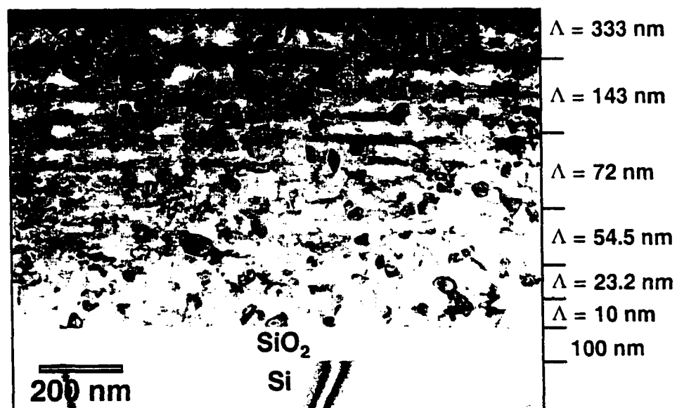
Figure 6. 32: Cross section TEM micrograph of a 1Nb/3Al multiple period sample annealed to 627°C at 40 °C/min.
