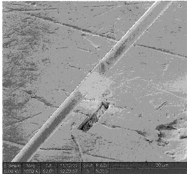
Figure 6-1: A cross-sectional FIB cut of a 10 μm diameter Al wire.
