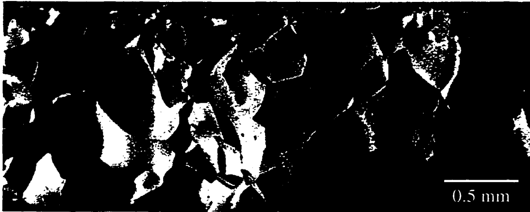
Figure 5.1 SEM micrograph of the fracture surface of S-doped Ni sample showing completely intergranular fracture.
