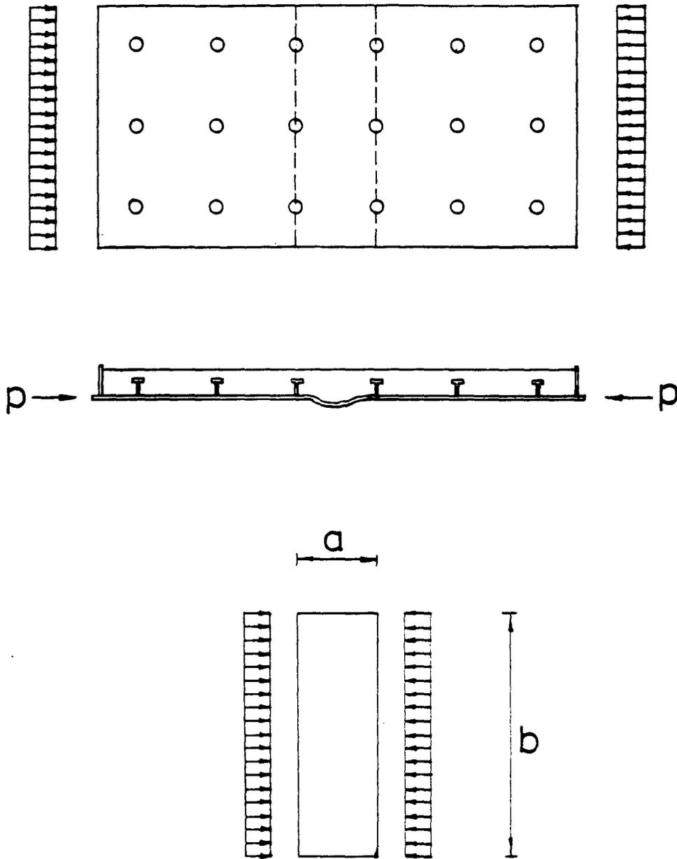
Figure 2 Local Buckling Between Anchor Rows
