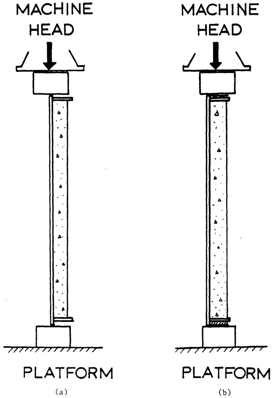
Figure 5 Loading Conditions of Panel Specimen
