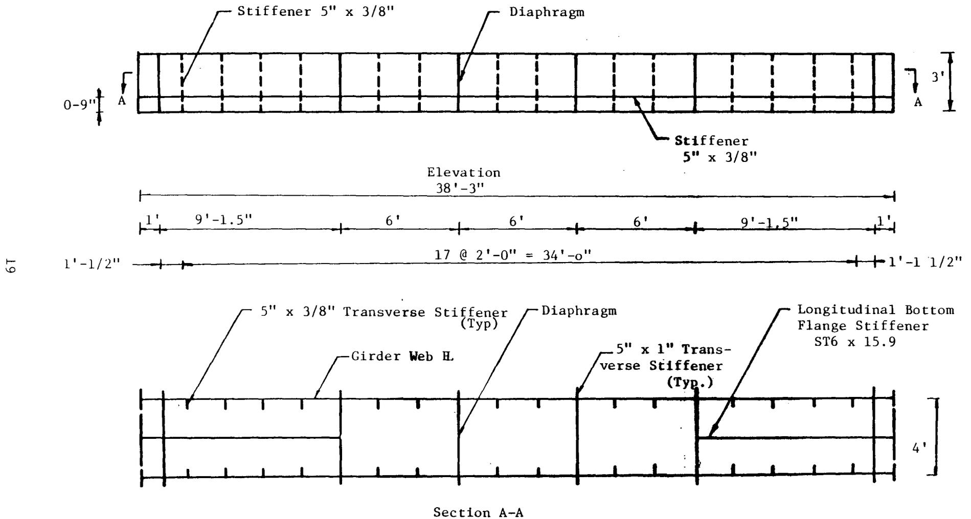
Figure 7 Box Girder Specimen
