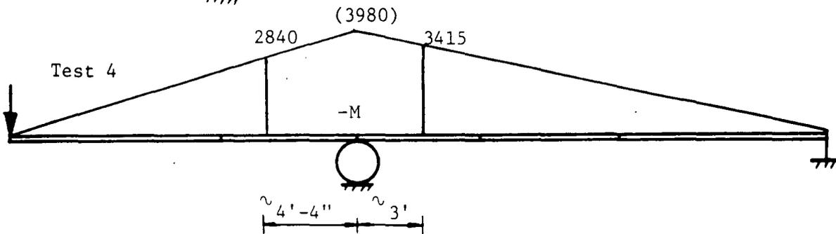
Figure 9 Support Locations and Moment Diagrams of Box Girder Specimen Tests
