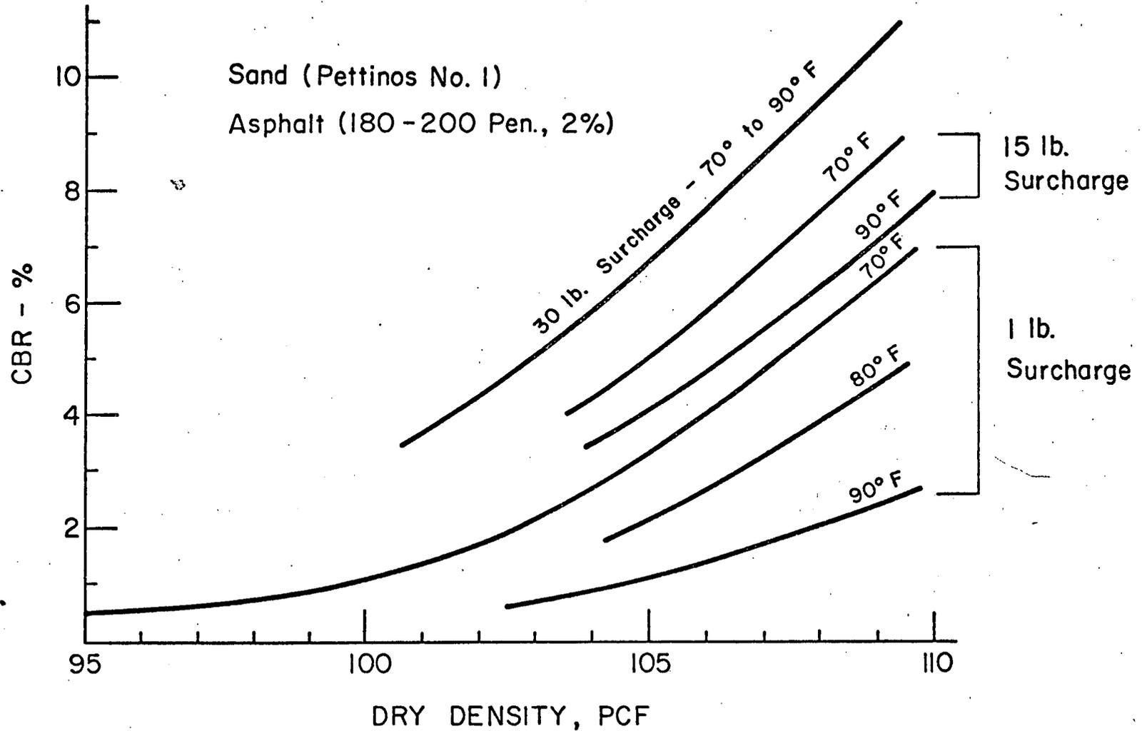
Fig. 4 Effect of Temperature and Surcharge on CBR of Sand-Asphalt Mixtures (from Winterkorn, 1968)
