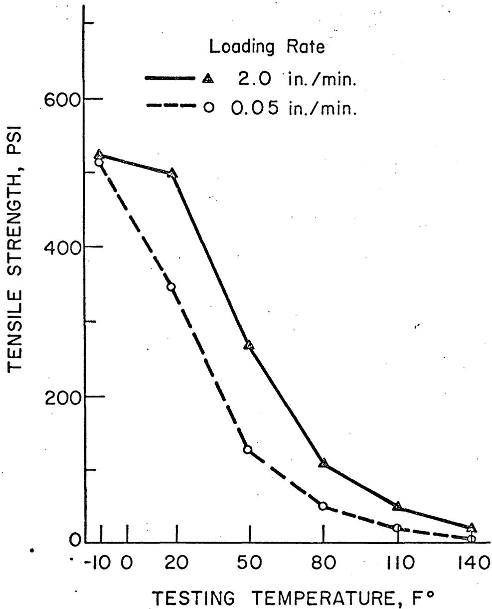
Fig. 2 Effect of Temperature on Tensile Strength of Bituminous Stabilized Materials (from Kennedy and Hudson, 1968)
