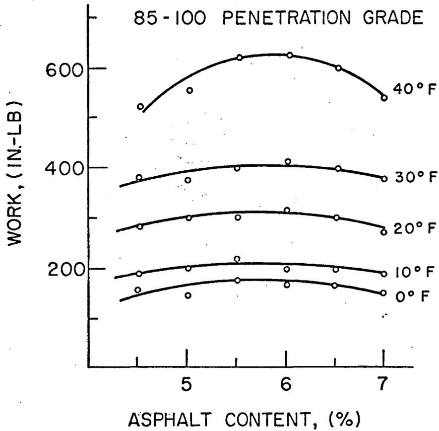
Fig. 3 Effect of Asphalt Content and Temperature on Work (from Breen and Stephens, 1966)
