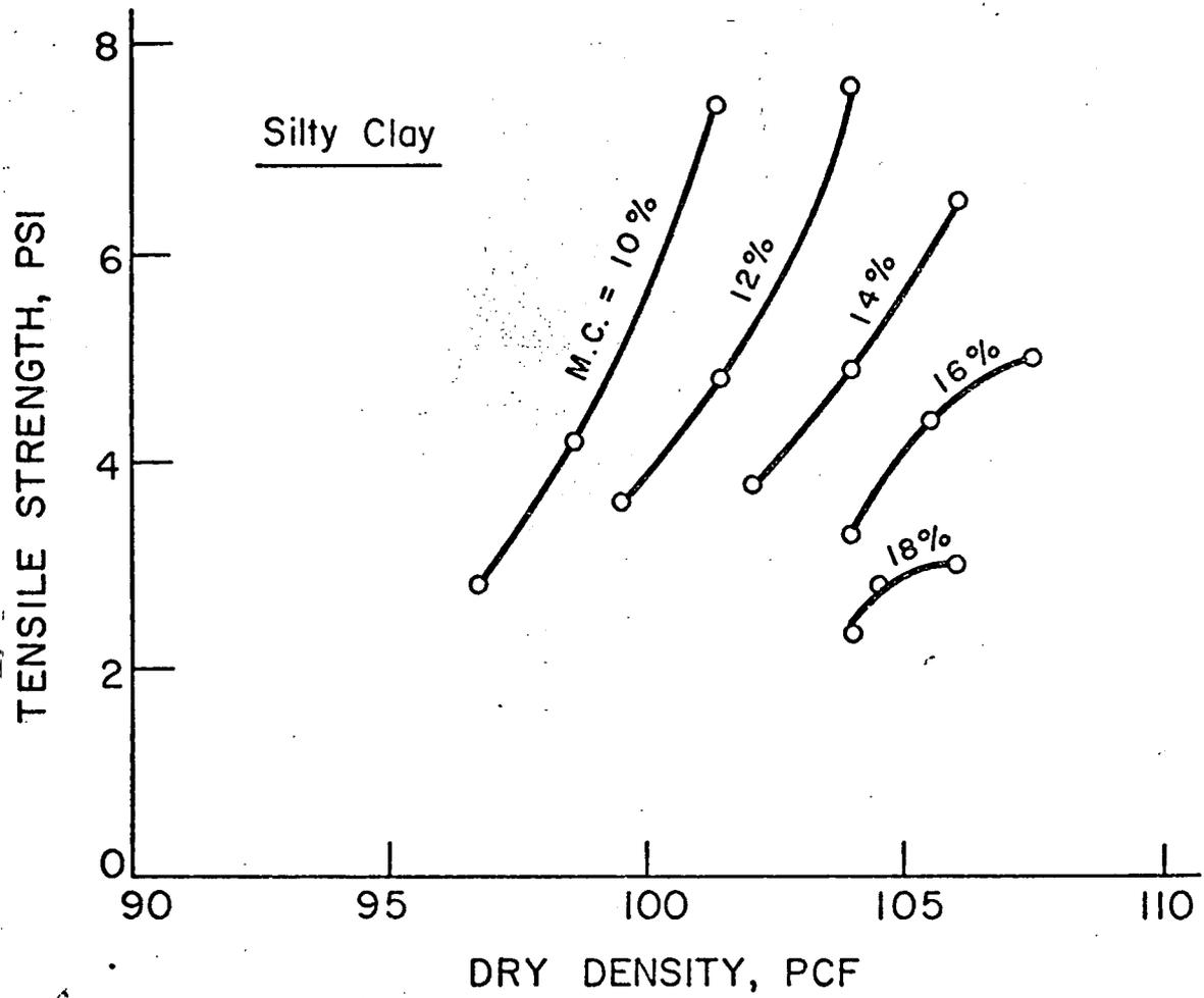
Fig. 1 Effect of Moisture Content and Dry Density on Tensile Strength (from Fang and Chen, 1971)
