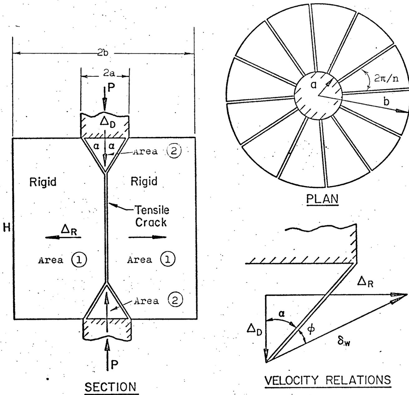
Fig. 4 Failure Mechanism of a Double Punch Test
