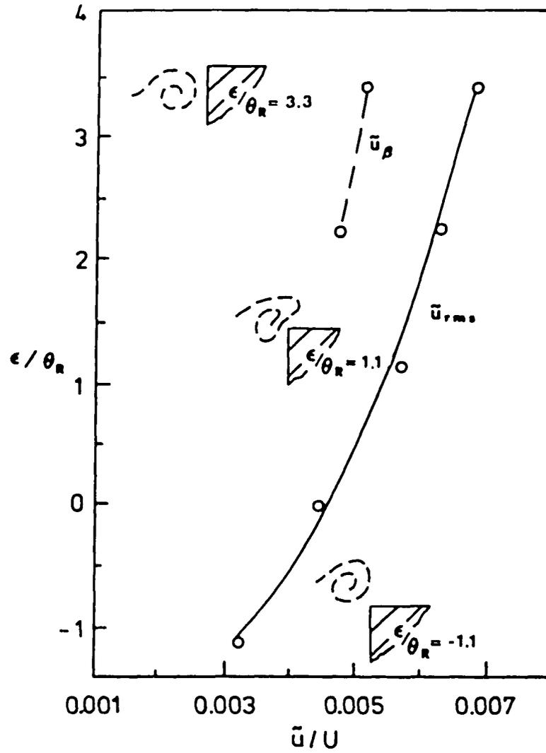
Figure 11: Root mean square of maximum longitudinal velocity fluctuation  $u_{rms}$  at separation ( $x' = 0$ ) as a function of corner offset for  $-1.1 \leq \epsilon / \theta_R \leq 3.3$ .
