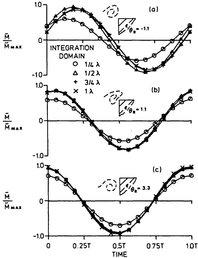
Figure 10: Fluctuating moment ( $\bar{M}$ ) about the intersection point ( $x/\lambda = 1$  and  $y/\lambda = 1$ ) as a function of size of integration domain for: (a)  $\epsilon/\theta_R = -1.1$ ; (b)  $\epsilon/\theta_R = 1.1$ ; and (c)  $\epsilon/\theta_R = 3.3$ .  $L/\theta_R = 31$ .  $\bar{M}_{max}$  has same value for all  $\epsilon/\theta_R$ .
