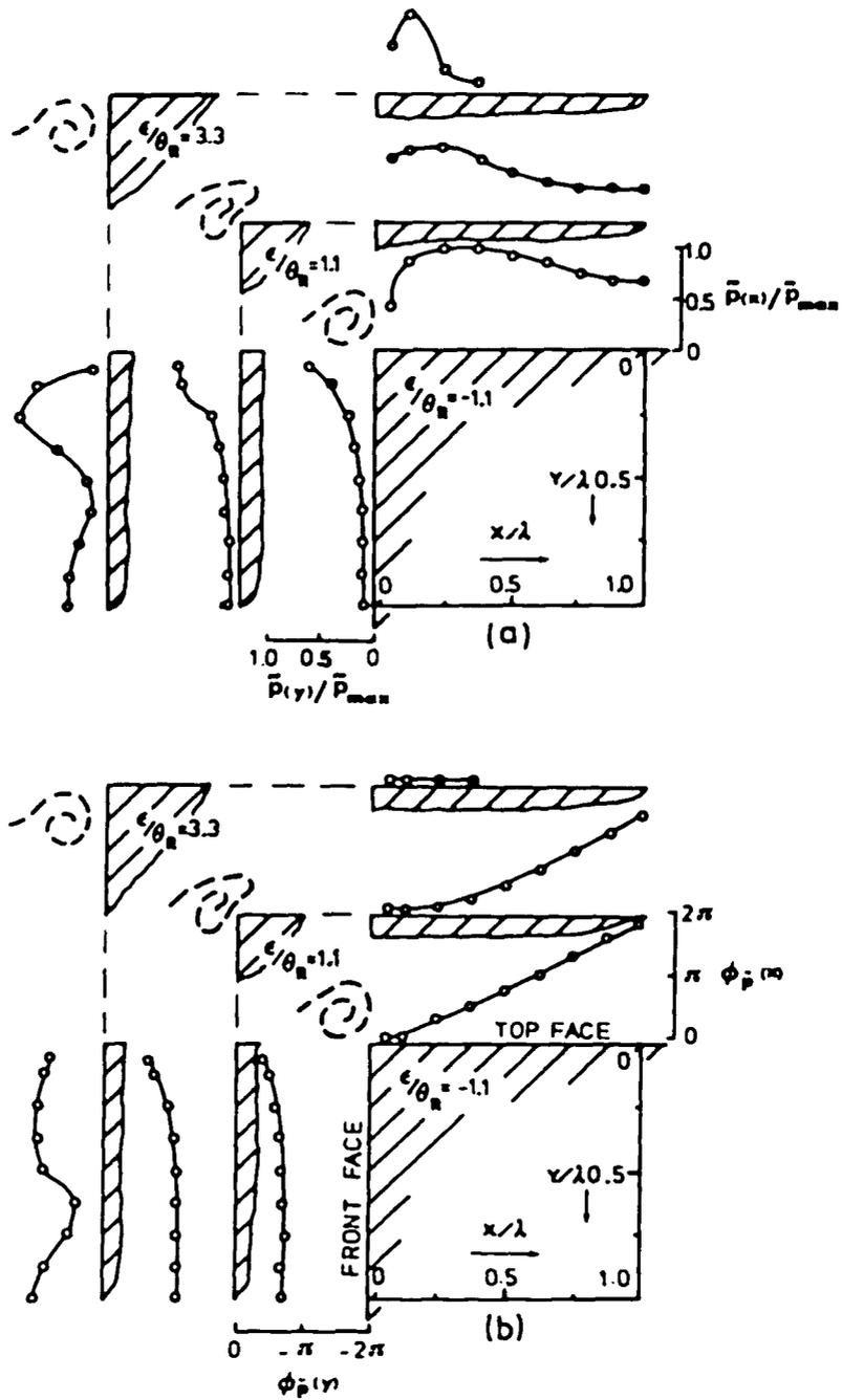
Figure 4: Distributions of: (a) time-averaged amplitudes; and (b) time-averaged phase of pressure. Both distributions shown along the top (x) and front (y) faces of the impingement corner for  $c/\theta_R = -1.1, 1.1$  and  $3.3$  at  $L/\theta_R = 31$ .
