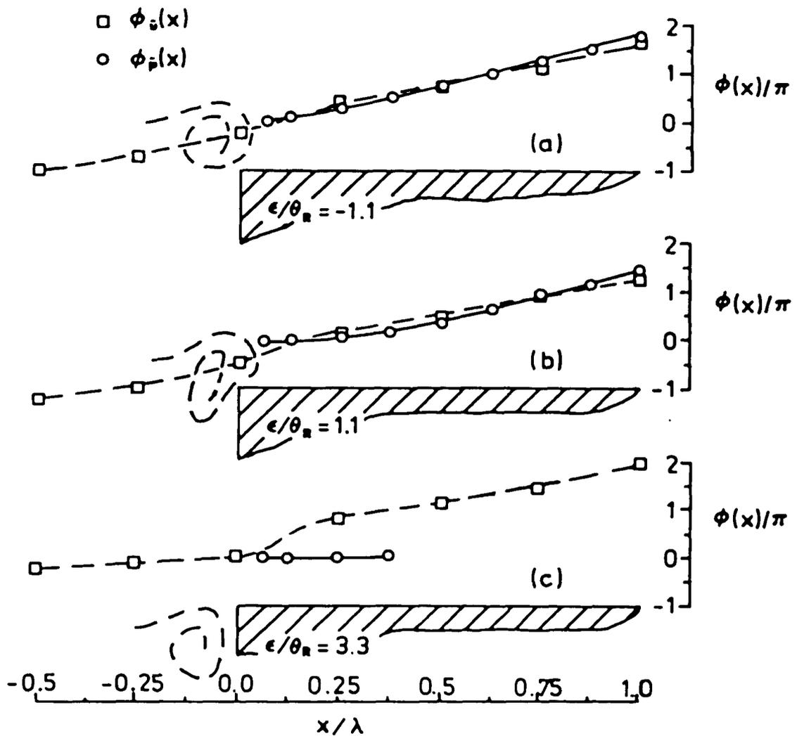
Figure 5: Streamwise phase distributions of: fluctuating velocity  $\phi_{\bar{u}}(x)$  taken along edge of shear layer; and fluctuating pressure  $\phi_{\bar{p}}(x)$  taken along wall.  $\epsilon/\theta_R = -1.1, 1.1$  and  $3.3$ .  $L/\theta_R = 31$ .
