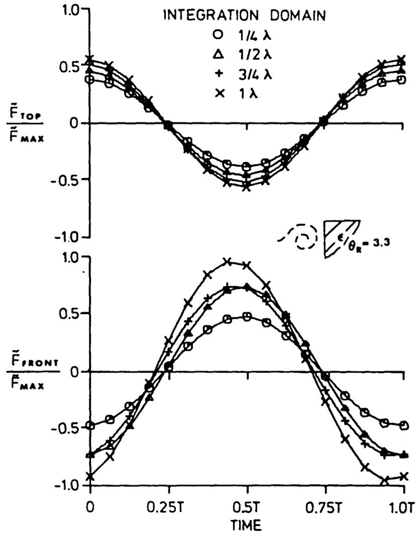
Figure 9c: Periodic forces ( $\bar{F}$ ) on top and front faces of the corner as a function of size of integration domain.  $\epsilon/\theta_R = 3.3$ ,  $L/\theta_R = 31$ .
