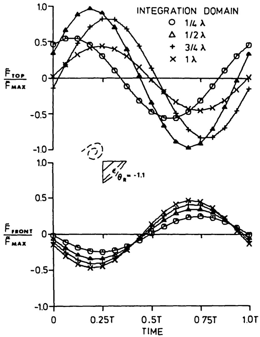
Figure 9a: Periodic forces ( $\bar{F}$ ) on top and front faces of the corner as a function of size of integration domain.  $\epsilon/\theta_R = -1.1$ ,  $L/\theta_R = 31$ .
