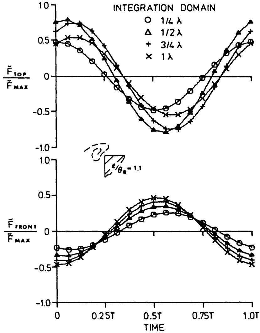
Figure 9b: Periodic forces ( $\bar{F}$ ) on top and front faces of the corner as a function of size of integration domain.  $\epsilon/\theta_R = 1.1$ ,  $L/\theta_R = 31$ .
