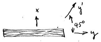
Intarolled section, le grains may be of The above shape when this is tested in tension or comp. along etther X or y direction, the max. shear developed in same sections. They may show the same strength in both directions, But the shearing strength magadiperent in x & y directions a tension specimen with white wash, cut along the y disettion may show the dyference 1 J-72<13
