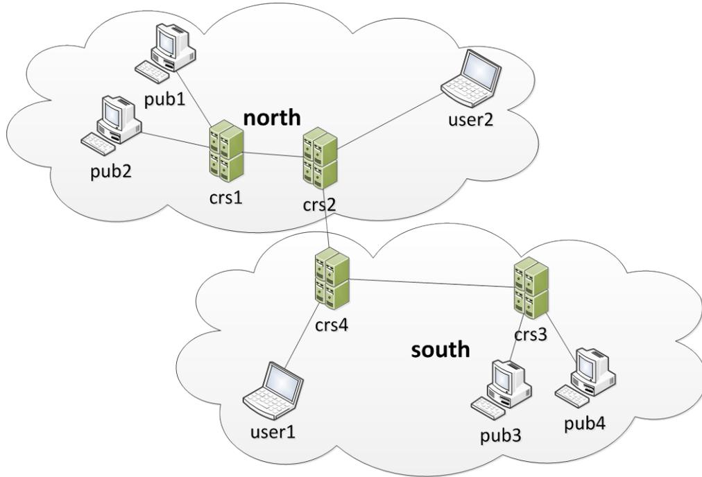
**Figure 7 Emulab Inter-domain experiments topology**
