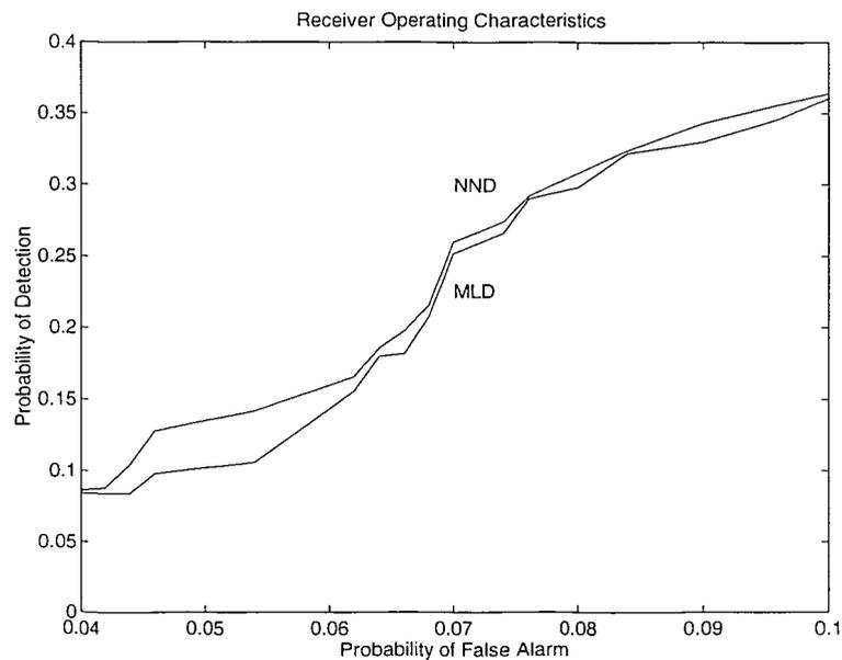
Figure 4.4:  $P_d$  versus  $P_f$  for uniform  $S_i$  and Generalized Gaussian  $W_i$  with  $k = 0.5$ ,  $\theta_0 = 1$ ,  $\mu = 0.5$ , and a network with 12 hidden nodes per layer and 2 hidden layers.
