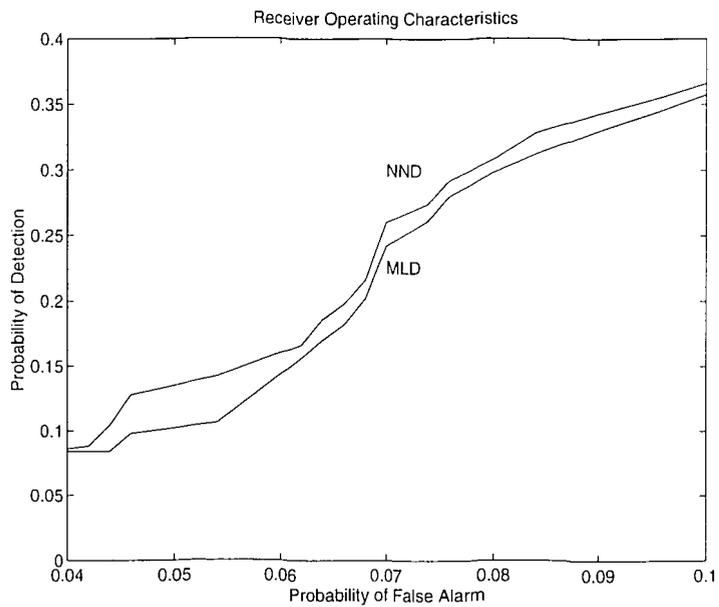
Figure 4.5:  $P_d$  versus  $P_f$  for uniform  $S_i$  and Generalized Gaussian  $W_i$  with  $k = 0.25$ ,  $\theta_0 = 1$ ,  $\mu = 0.5$ , and a network with 18 hidden nodes and 1 hidden layer.
