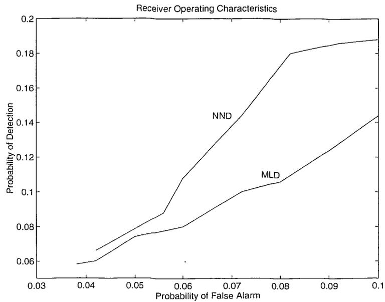
Figure 4.2:  $P_d$  versus  $P_f$  for Cauchy  $S_i$  and  $W_i$ ,  $\theta_0 = 0.5$ ,  $\mu = 2.0$ , and a network with 5 hidden nodes and 1 hidden layer.
