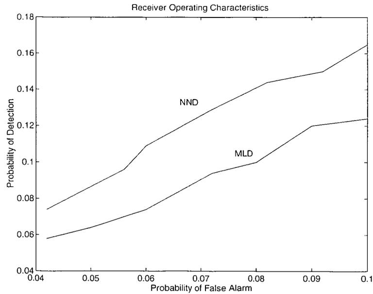
Figure 4.3:  $P_d$  versus  $P_f$  for Cauchy  $S_i$  and  $W_i$ ,  $\theta_0 = 0.3$ ,  $\mu = 2.0$ , and a network with 4 hidden nodes and 1 hidden layer.
