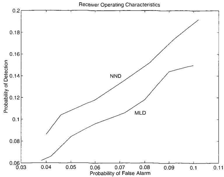
Figure 4.1:  $P_d$  versus  $P_f$  for Cauchy  $S_i$  and  $W_i$ ,  $\theta_0 = 0.5$ ,  $\mu = 2.0$ , and a network with 4 hidden nodes and 1 hidden layer.
