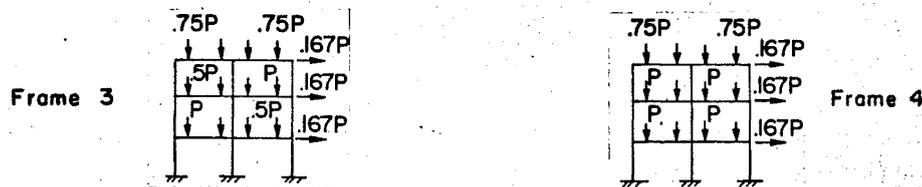
FIG. 2 LOADING CONDITION AT ULTIMATE LOAD
