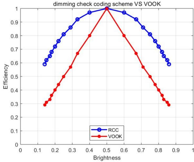
Fig.1 dimming check coding scheme VS VOOK, data bits length K=4, filler bits length M=1 to 10.
