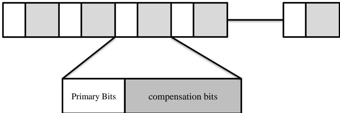
Fig.3 the frame structure of proposed encoded signal
