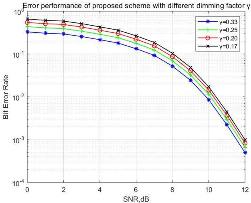
Fig.6 error performance of proposed scheme with different dimming factor  $\gamma$
