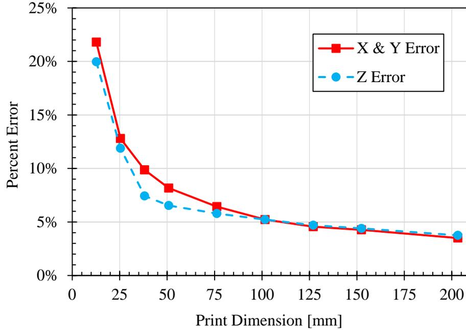
Figure 4: Printer Bleed Correlation with Print Dimension
