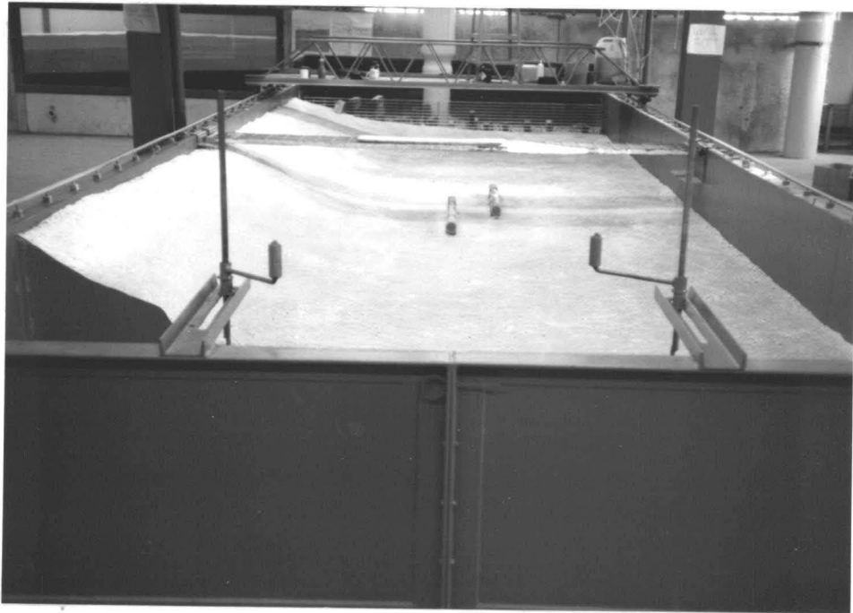
Photograph 1: Modeling tank with intakes, looking upstream toward headbox.
