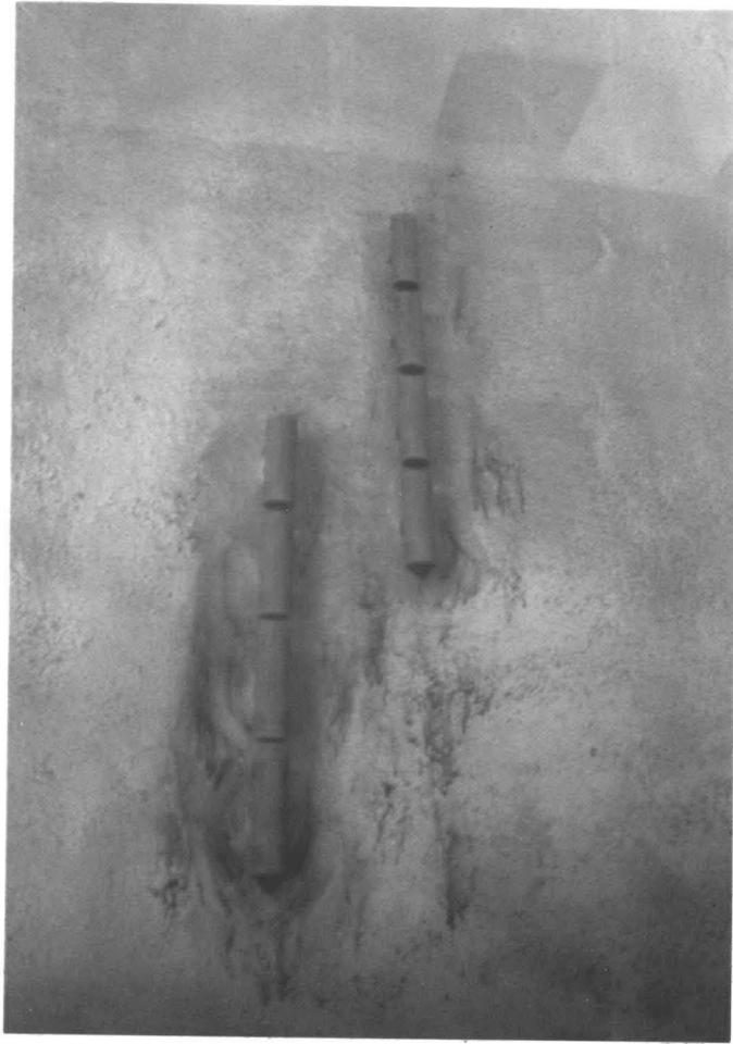
Photograph 3: Potassium permanganate crystals in the model with flow from bottom towards top, showing bottom currents.
