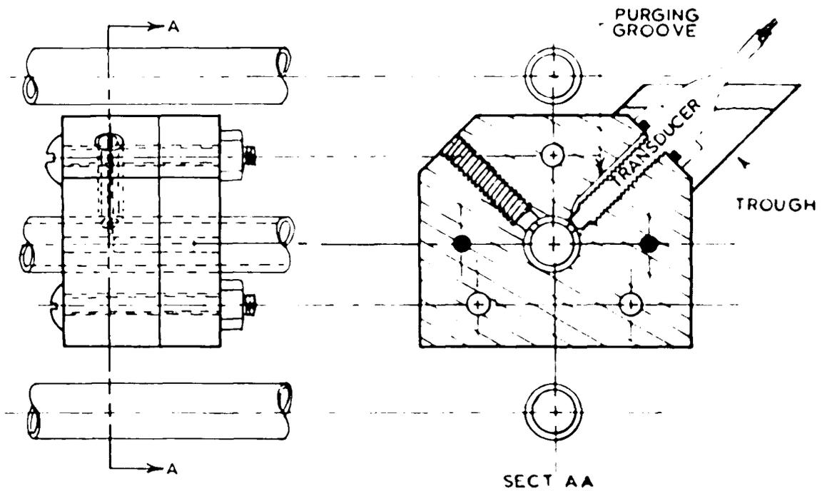
Fig. 5 Transducer block
