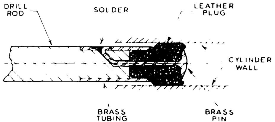
Fig. 7 Details of 3.18mm piston
