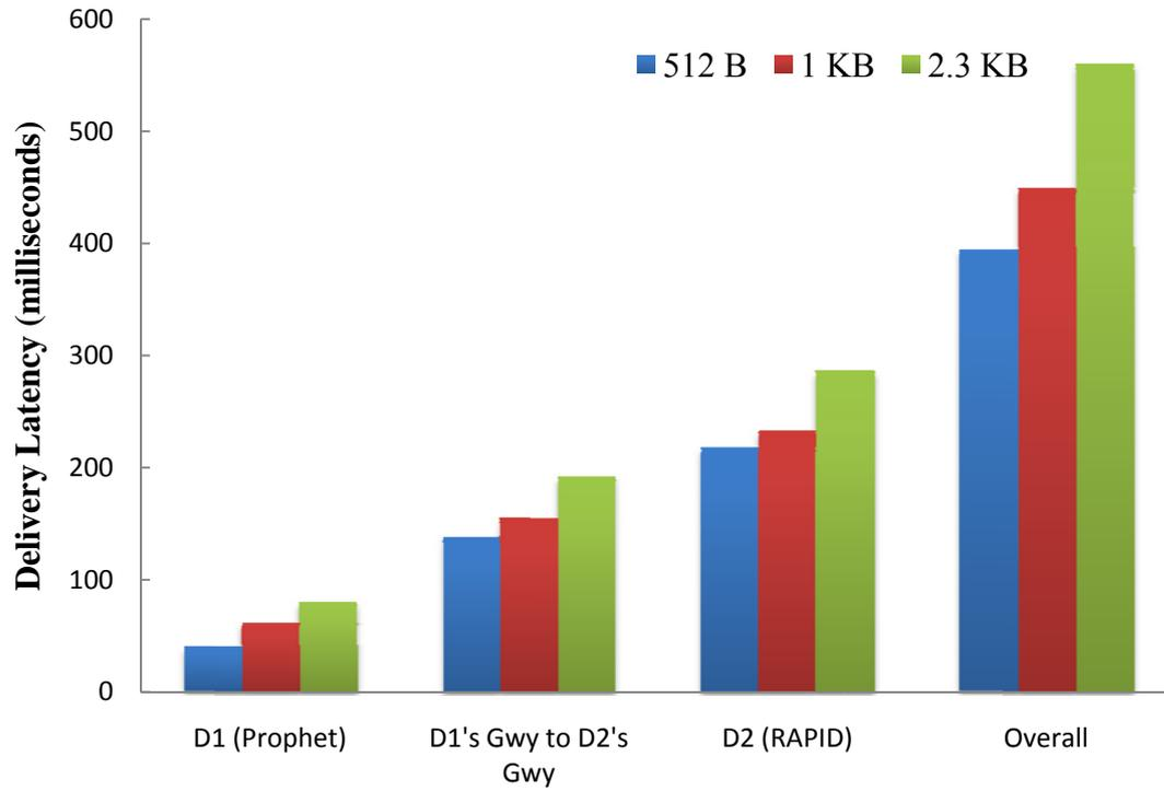
**Figure 6: Delivery Latency of One domain hop**
