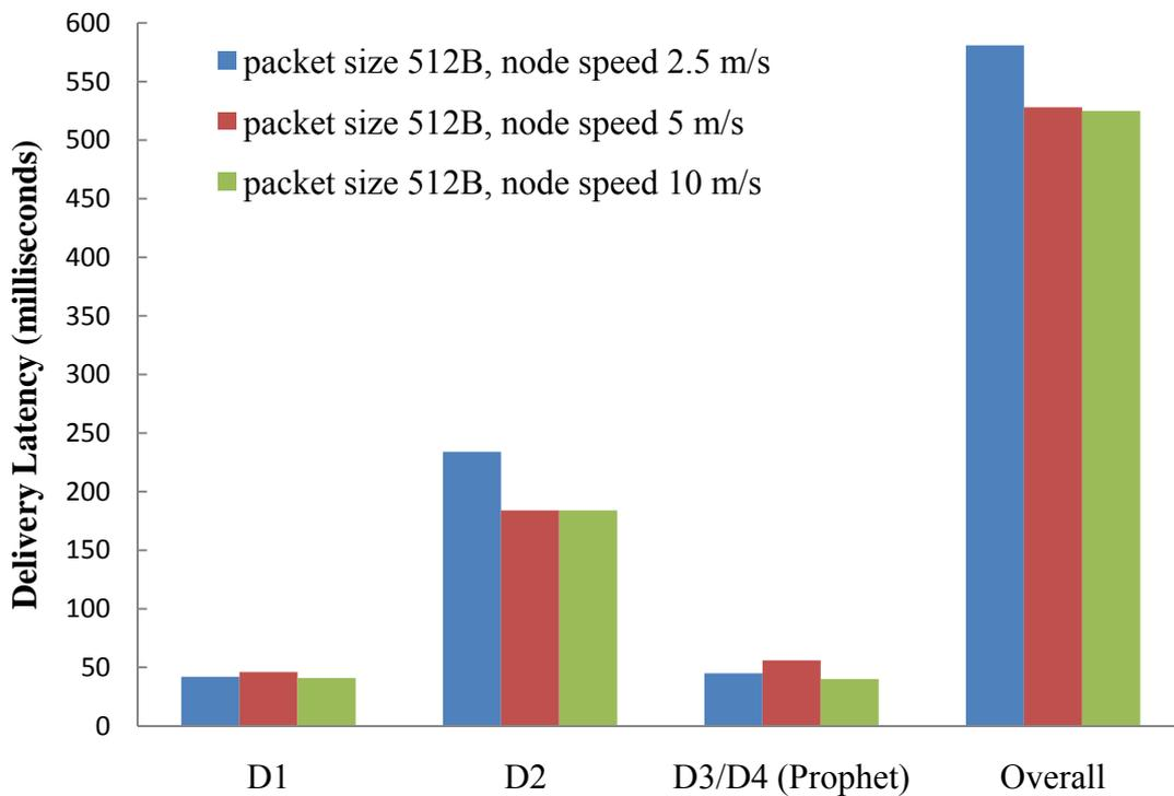
**Figure 12: Delivery Latency of Two domains hop for 512B with different node speed**
