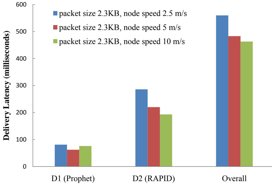
**Figure 11: Delivery Latency of One domain hop for 2.3 KB with different node speed**
