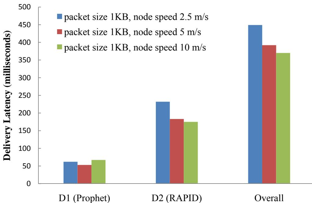
**Figure 10: Delivery Latency of One domain hop for 1 KB with different node speed**
