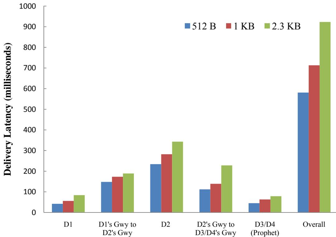
**Figure 7: Delivery Latency of Two domains hop**
