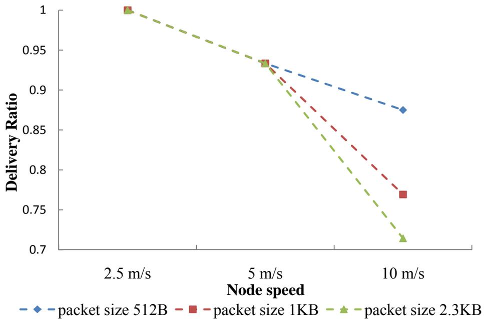
**Figure 18: Delivery Ratio of one domain hop vs Node speed**
