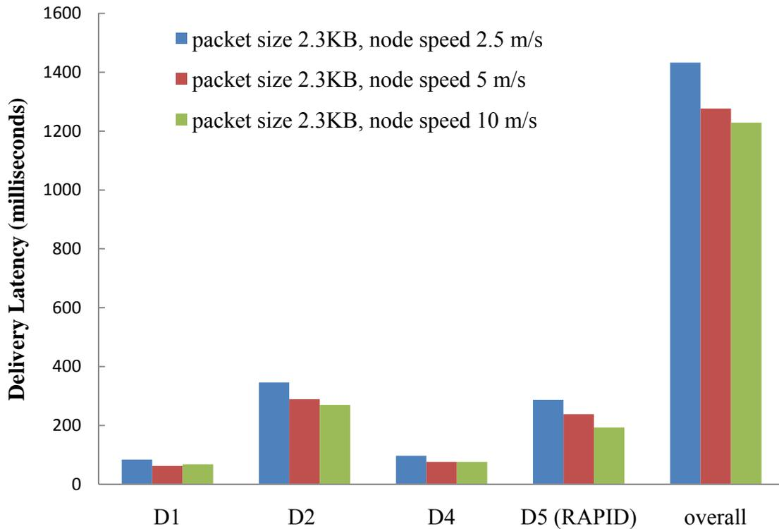
**Figure 17: Delivery Latency of Three domains hop for 2.3KB with different node speed**
