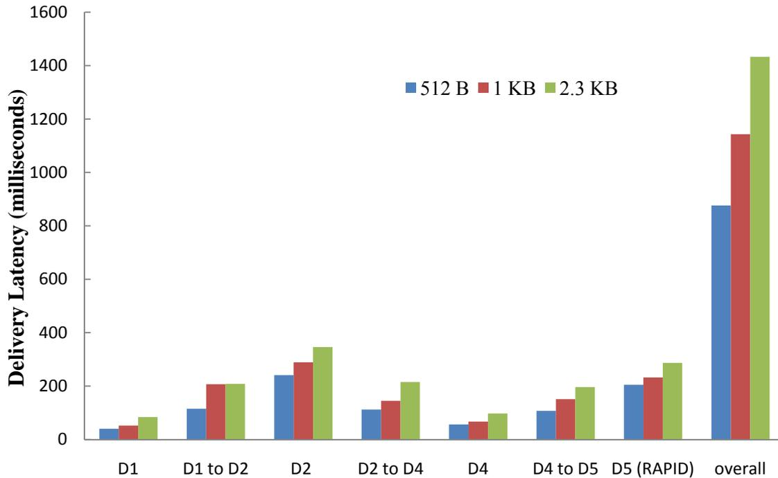
**Figure 8: Delivery Latency of Three domains hop**
