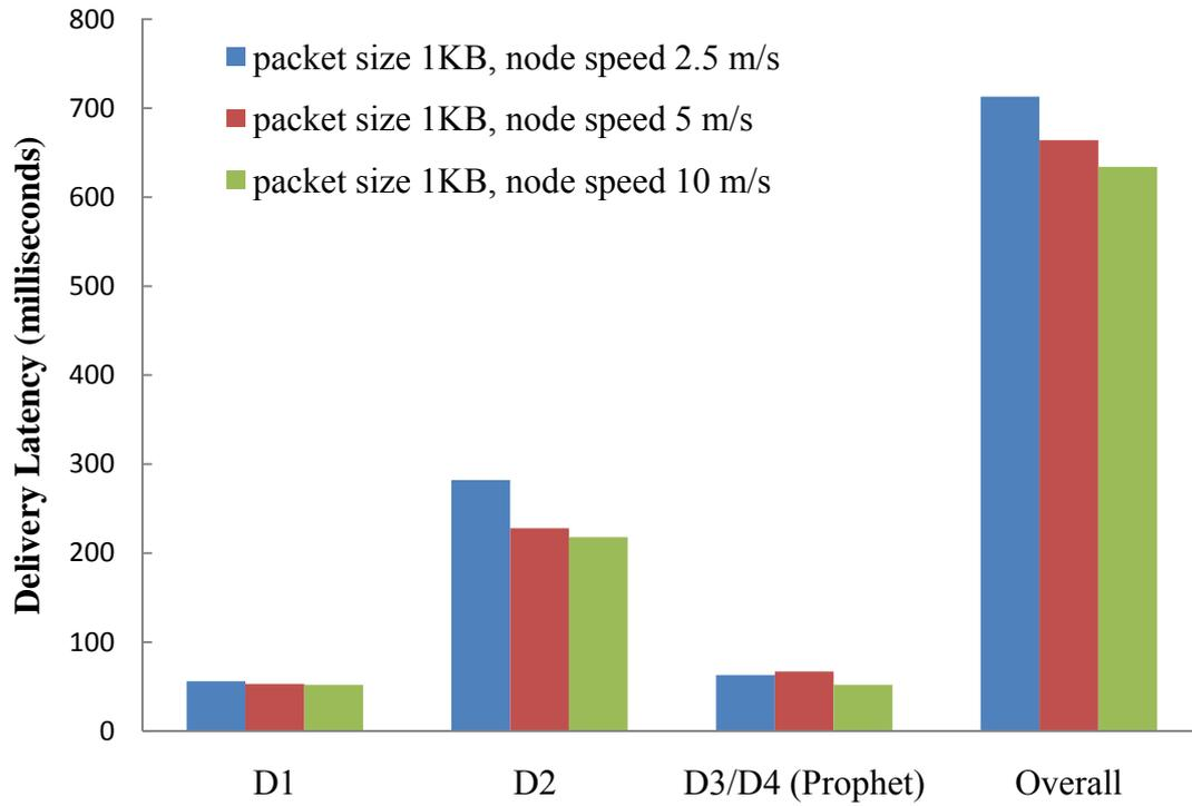
**Figure 13: Delivery Latency of Two domains hop for 1KB with different node speed**
