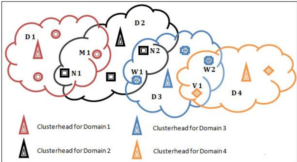
**Figure 4: More detail about GBIR in complex inter-domain routing scenario**
