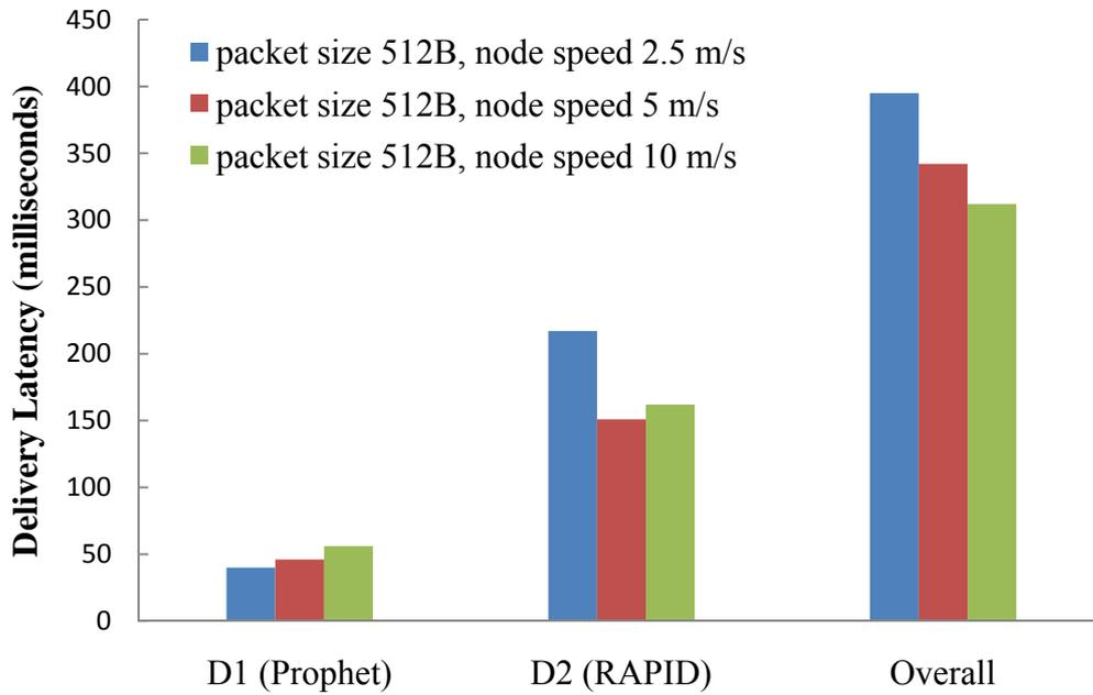
**Figure 9: Delivery Latency of One domain hop for 512 B with different node speed**
