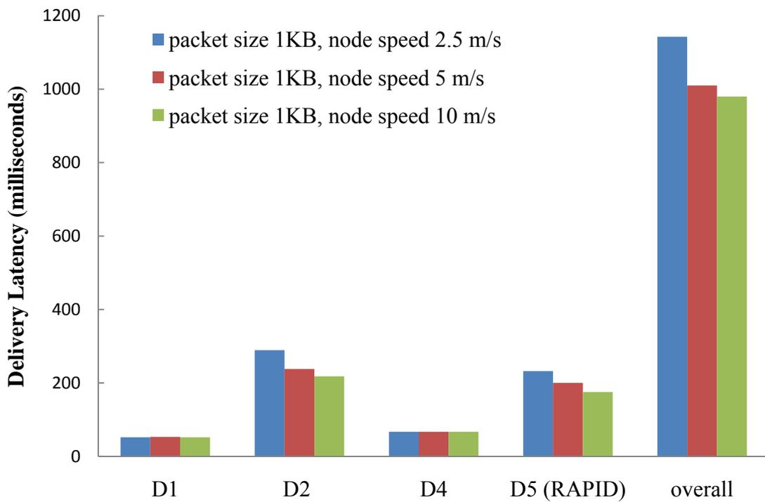
**Figure 16: Delivery Latency of Three domains hop for 1KB with different node speed**
