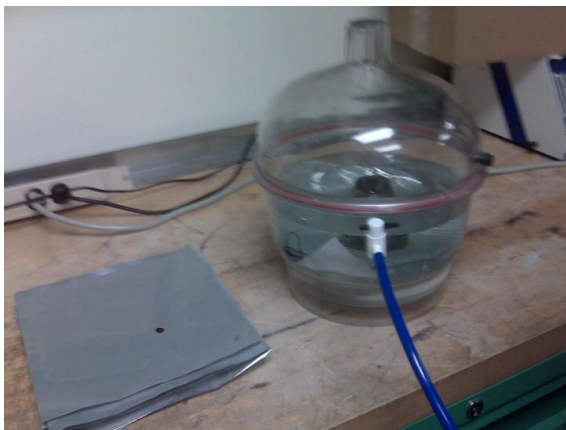
Figure 3 Bubble Leak Test Station
