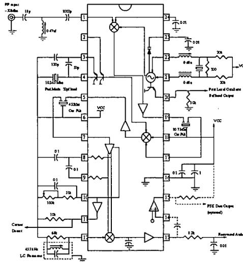
Figure 4.2: Application circuit for MC3362
