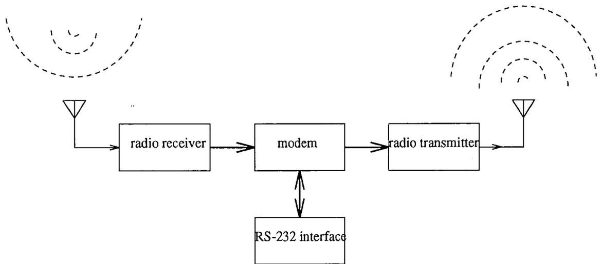
Figure 1.1: Radio Modem Block Diagram
