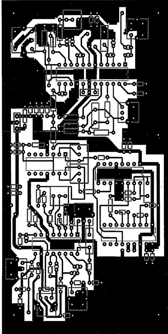
Figure 1.2: Radio Modem Printed Circuit Board
