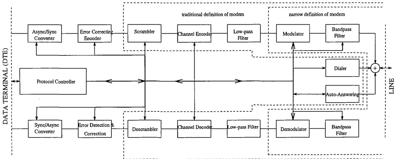
Figure 2.1: Components of a *full*, a *traditional*, and a *narrowly* defined modem
