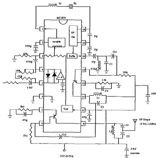
Figure 3.2: Application Circuit for MC2833
