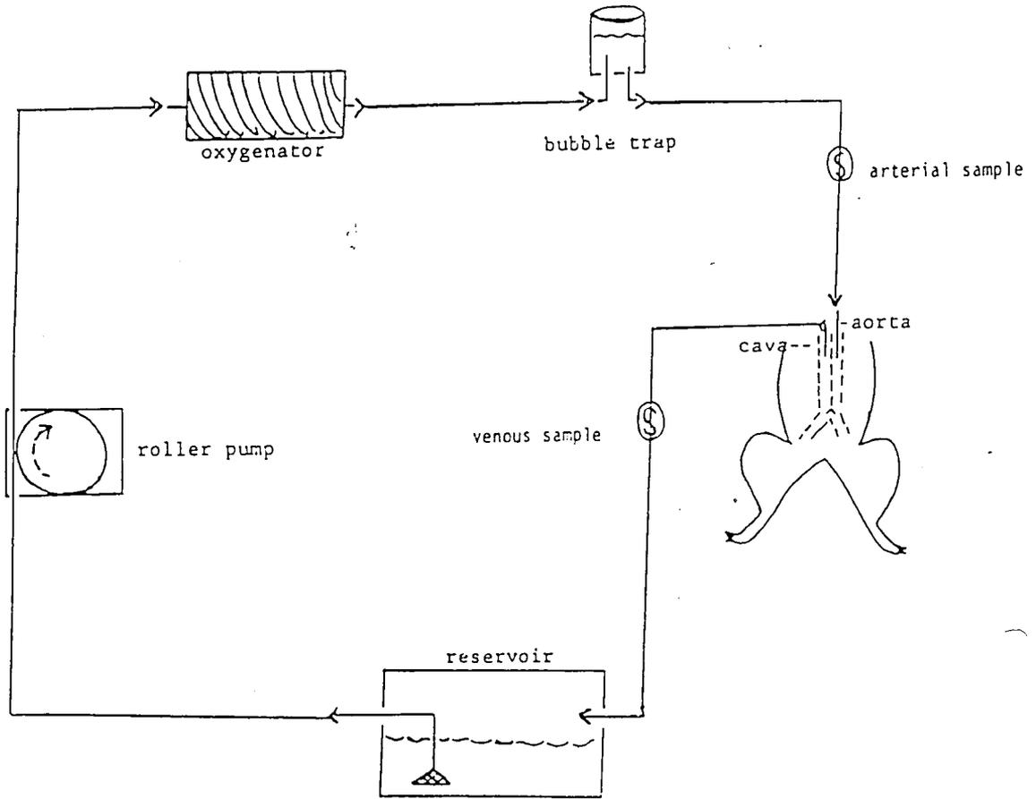
A schematic of the isolated, perfused rat hindlimb preparation.
