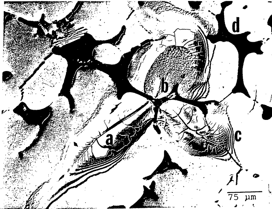
Fig. 4: Micrograph of an as-cast AA2090 Al-Li alloy illustrating the presence of: (a) solidification cracking, (b) dendrite tip fracture, (c) coring and (d) interdendritic porosity.
