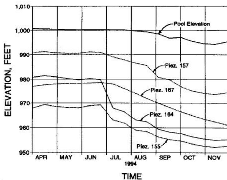
**Figure 8: Piezometer Readings 1994 (Bingham et al. 1996)**
