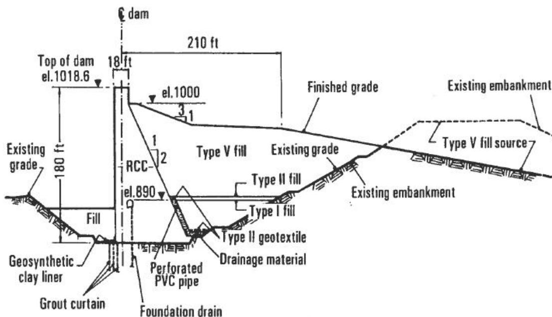
*Typical Section of RCC Replacement Dam*
